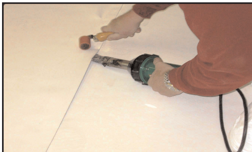
Approved Hand Held Welder with silicone roller, assorted tips and #12 power cord (power supply: 115 volts, 15 amp, 1800 watts single phase)
