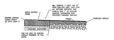
Lap Joint Detail - Asphalt Pavement
