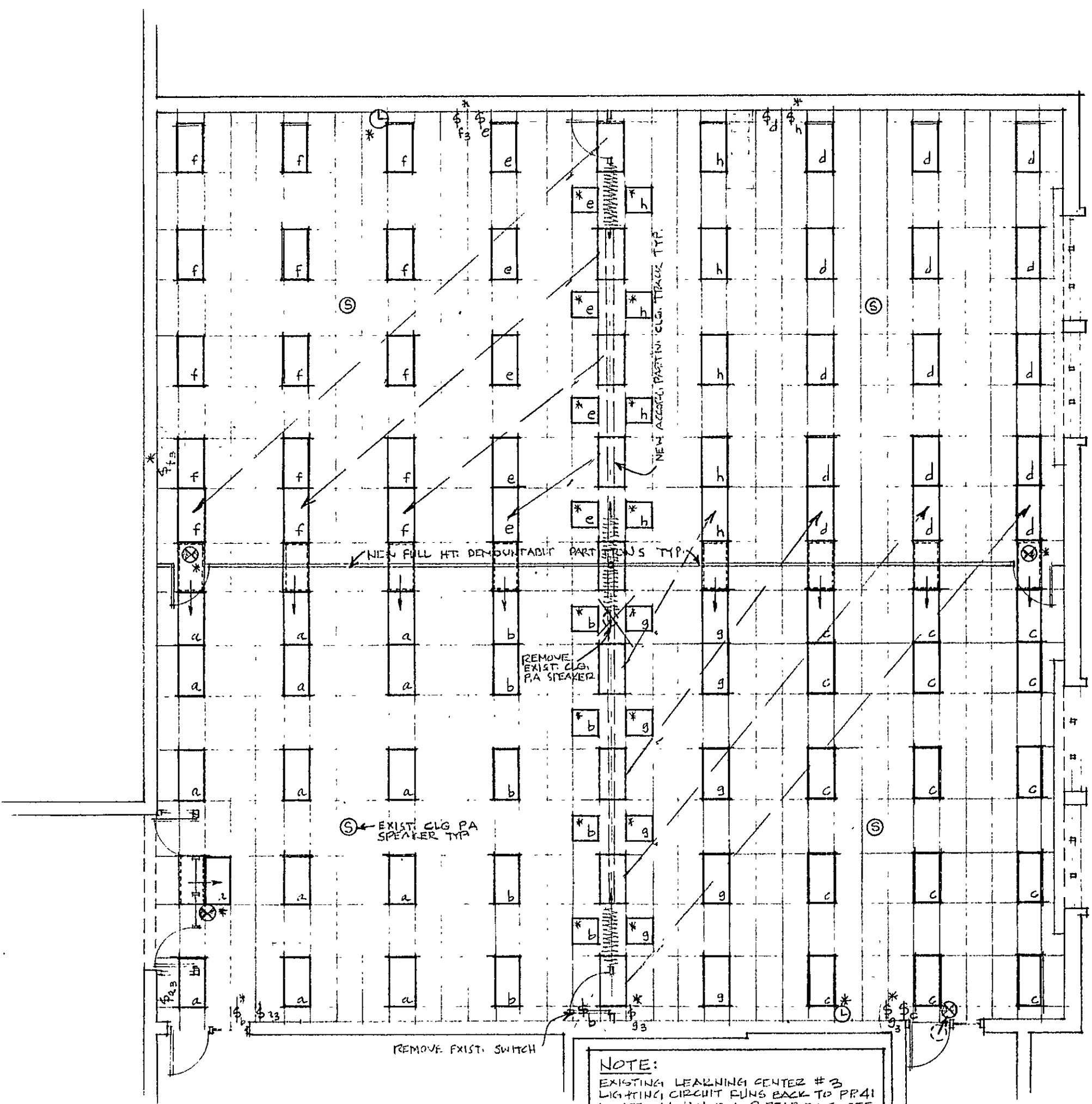
REVISED CEILING/LIGHTING PLAN BRUMMITT ELEMENTARY LEARNING CENTER #3 1/8"=1'-0"
